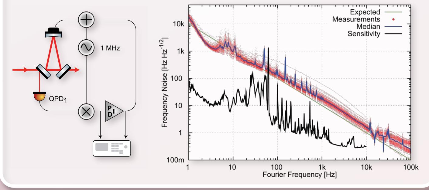
100 automated measurements of the NPRO frequency noise [2,5]
